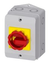
SENTRON, Switch disconnector 3LD, emergency switching-off switch, 3- pole, lu: 32 A, operating power / at AC-23 A 400 V: 11.5 kW, molded-plastic encapsulation for inch screw connection 4 NO, rotary operating mechanism, red/yellow
