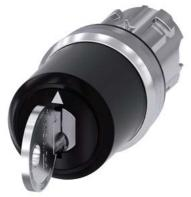
Key-operated switch IKON, 22 mm, round, metal, shiny, lock number 360012K1, with 2 keys, 3 switch positions I-O-II, latching, actuating angle  $2x45^{\circ}$ , 10:30h/12h/13:30h, Key removal I+O+II, with laser labeling, upper case
