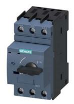
Circuit breaker size S00 for starter combination Rated current 6.3 A N-release 82 A screw terminal Standard switching capacity
