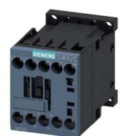
power contactor, AC-3, 16 A, 7.5 kW / 400 V, 4-pole, 24 V DC, main contacts: 2 NO + 2 NC, screw terminal, size: S00
