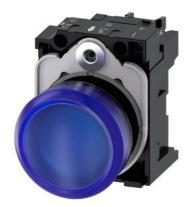
Indicator lights, 22 mm, round, plastic, blue, lens, smooth, with holder, LED module, with integrated LED 24 V AC/DC, screw terminal
