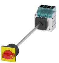
Load disconnector 3LD3, lu 16 A Main switch 3-pole + N Rated operating capacity at AC-23 A at 400V 7.5kW floor mounting Basic switch with door coupling Central hole mounting 22.5mm Toggle drive red / yellow 48x48 mm with auxiliary switch 10E + 1S
