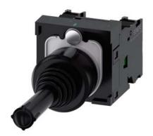
Coordinate switch, 22 mm, round, plastic, black, 2 switch positions, horizontal, momentary contact type, without mechanical interlocking in O position, with holder, 1 NO, 1 NO, screw terminal, Z=20-unit packaging
