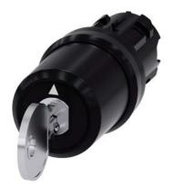
key-operated switch Siemens, 22 mm, round, plastic, lock number SSG10, with 2 keys, 3 switch positions I>O<II, momentary contact on the left, latching on the right, actuating angle 2x45°, 10:30h/12h/13:30h, key removal O, with laser labeling, upper case
