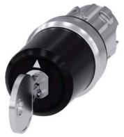
key-operated switch Siemens, 22 mm, round, metal, shiny, lock number SSG10, with 2 keys, 3 switch positions I>O<II, momentary contact on the left, latching on the right, actuating angle  $2x45^{\circ}$ , 10:30h/12h/13:30h, key removal O
