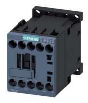
power contactor, AC-3e/AC-3, 12 A, 5.5 kW / 400 V, 3-pole, 24 V DC, 0.7-1.25\* Us, with integrated suppressor diode, auxiliary contacts: 1 NO, screw terminal, size: S00, suitable for PLC outputs, not expandable with auxiliary switch
