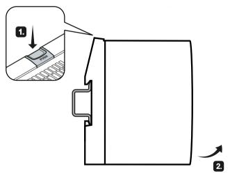
Figure 5-2 Removing from a DIN rail
