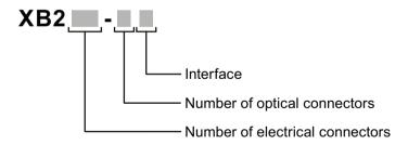
Interfaces of devices with optical connectors:
