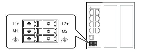
Figure 6-1 Position of the power supply, for example on the SCALANCE XB213-3
