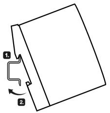
Figure 5-1 DIN rail mounting
