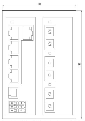
Figure 9-2 Width and height based on the example of the SCALANCE XB205-3
