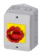
SENTRON, Switch disconnector 3LD, emergency switching-off switch, 3- pole, lu: 16 A, operating power / at AC-23 A 400 V: 7.5 kW, Molded plastic encapsulation for inch cable gland, 1 NC, 1 NO, rotary operating mechanism, red/yellow
