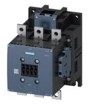
power contactor, AC-3e/AC-3 300 A, 160 kW / 400 V, AC (50-60 Hz) / DC Uc: 200-277 V PLC input 24 V DC 3-pole, auxiliary contacts 2 NO + 2 NC drive: electronic main circuit: busbar control and auxiliary circuit: screw terminal
