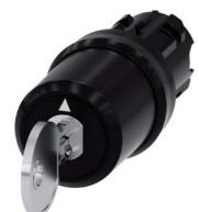
key-operated switch Siemens, 22 mm, round, plastic, lock number SSG10, with 2 keys, 3 switch positions I>O<II, momentary contact on the left, latching on the right, actuating angle 2x45°, 10:30h/12h/13:30h, key removal O
