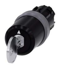
Key-operated switch BKS, 22 mm, round, plastic with metal front ring, special lock, with 2 keys, 3 switch positions I>O<II, momentary contact type, actuating angle  $2x45^{\circ}$ , 10:30h/12h/13:30h, key removal O, Note: BKS locking systems E1 - E25 supplied without key
