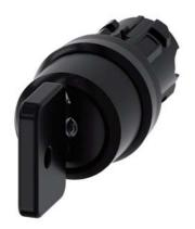
Key-operated switch O.M.R, 22 mm, round, plastic, lock number 73034, black, with 2 keys, 3 switch positions I-O-II, latching, actuating angle 2x45°, 10:30h/12h/13:30h, Key removal I+O+II, with laser labeling, lower case
