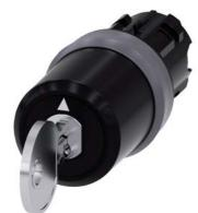
key-operated switch Siemens, 22 mm, round, plastic with metal front ring, lock number SSG10, with 2 keys, 3 switch positions I>O<II, momentary contact on the left, latching on the right, actuating angle 2x45°, 10:30h/12h/13:30h, key removal O, with laser labeling, inscription or symbol customer-specific selection with SIRIUS ACT configurator (CIN)
