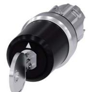
key-operated switch Siemens, 22 mm, round, metal, shiny, lock number SSG10, with 2 keys, 3 switch positions I>O<II, momentary contact on the left, latching on the right, actuating angle 2x45°, 10:30h/12h/13:30h, key removal O, Z=50-unit packaging
