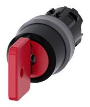
Key-operated switch O.M.R, 22 mm, round, plastic with metal front ring, lock number 73037, red, with 2 keys, 3 switch positions I-O-II, latching, actuating angle 2x45°, 10:30h/12h/13:30h, key removal O, Z=50-unit packaging
