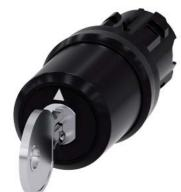
key-operated switch Siemens, 22 mm, round, plastic, lock number SSG10, with 2 keys, 3 switch positions I>O<II, momentary contact on the left, latching on the right, actuating angle 2x45°, 10:30h/12h/13:30h, key removal II
