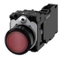
Illuminated pushbutton, 22 mm, round, plastic, red, pushbutton, flat, momentary contact type, with holder, 1 NO+1 NC, LED module with integrated LED 24 V AC/DC, screw terminal
