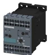
Timing relay, electronic Multifunction, 8 functions 1 change-over contact 24 V AC/DC, 100 AC to 127 V at 50/60 Hz AC 0.05 s to 100 h Overall width 45 mm Spring-type terminal
