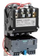
Non-reversing motor starter Size 1 Three phase full voltage Solid-state overload relay OLRelay amp range 0.75-3.4A 24VAC 50-60HZ coil Combination type No enclosure
