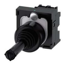
Coordinate switch, 22 mm, round, plastic, black, 2 switch positions, vertical latching, without mechanical interlocking, in O position, with holder, 1 NO, 1 NO, screw terminal, Z=20-unit packaging
