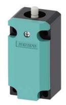
Basic switch for position switch 3SE5112 Metal enclosure, according to EN 50041 40 mm, 1 x (M20x 1.5) 1 NO/2 NC slow-action contacts with make-before-break without actuator head
