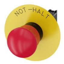
EMERGENCY STOP mushroom-type actuator, 22 mm, round, plastic, red, 40 mm, positive latching, according to EN ISO 13850, rotate-to-unlatch, with yellow backing plate, inscription: NOT-HALT, with holder, 1 NC, screw terminal
