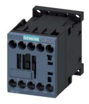
power contactor, AC-3e/AC-3, 7 A, 3 kW / 400 V, 3-pole, 24 V DC, auxiliary contacts: 1 NO, screw terminal, size: S00,
