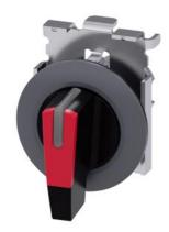
Selector switch, illuminable, 30 mm, round, Metal, matte, red, selector switch, long, front ring for flush installation, 3 switch positions I>O<II, momentary contact type, actuating angle  $2x45^{\circ}$ , 10:30h/12h/13:30h, with laser labeling, lower case
