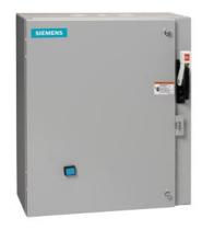
Non-reversing motor starter, Size 1, Three phase full voltage, Solid-state overload relay, OLR amp range 3-12A, 240V 50Hz / 277V 60Hz coil, Combination type, 30A non-fusible disconnect, Enclosure NEMA type 1, Indoor general purpose use, Extra-wide enclosure
