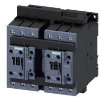
reversing contactor assembly, AC-3e/AC-3, 80 A, 37 kW / 400 V, 3-pole, 110 V AC, 50 Hz / 120 V, 60 Hz, screw terminal, electrical and mechanical interlock, auxiliary contacts: 2 x 1 NO
