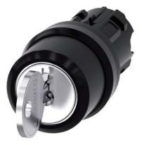
RONIS key-operated switch, 22 mm, round, plastic, lock number SB30, with 2 keys, 3 switch positions I>O<II, momentary contact on the left, latching on the right, actuating angle 2x45°, 10:30h/12h/13:30h, Key removal O+II, possible special locks: SB31, 421, 455, with laser labeling, inscription or symbol Customer-specific selection with SIRIUS ACT configurator (CIN)
