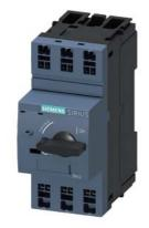
Circuit breaker size S00 for starter combination Rated current 0.4 A N-release 5.2 A Spring-type terminal Standard switching capacity
