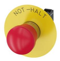
EMERGENCY STOP mushroom-type actuator, 22 mm, round, metal, shiny, red, 40 mm, positive latching, according to EN ISO 13850, pull-to-unlatch mechanism, with yellow backing plate, inscription: NOT-HALT, with holder, 1 NC, spring-type terminal
