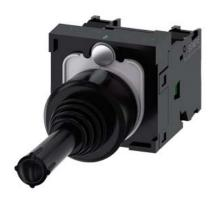
Coordinate switch, 22 mm, round, plastic, black, 2 switch positions, horizontal, momentary contact type, without mechanical interlocking in O position, with holder, 1 NO, 1 NO, screw terminal
