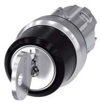
RONIS key-operated switch, 22 mm, round, metal, shiny, lock number SB30, with 2 keys, 3 switch positions >O<II, momentary contact on the left, latching on the right, actuating angle  $2x45^{\circ}$ , 10:30h/12h/13:30h, key removal O, possible special locks: SB31, 421, 455, Z=50-unit packaging
