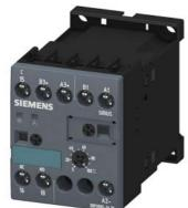
Timing relay, electronic Multifunction, 8 functions 1 change-over contact 24 V AC/DC, 200 to 240 V AC at 50/60 Hz AC 0.05 s to 100 h Overall width 45 mm screw terminal
