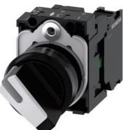
Selector switch, illuminable, 22 mm, round, plastic, white, selector switch, short, 2 switch positions O-I, latching, 10:30h/13:30h, with holder, 1 NO, screw terminal, Z=20-unit packaging
