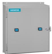
Duplex starter w/o alternator, Size 0, Three phase full voltage, Solid-state overload relay, OLR amp range 3-12A, 240V 50Hz / 277V 60Hz coil, Non-combination type, Enclosure NEMA type 12, Dust/drip proof for indoors
