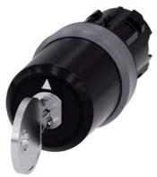
key-operated switch Siemens, 22 mm, round, plastic with metal front ring, lock number SSG10, with 2 keys, 3 switch positions I>O<II, momentary contact on the left, latching on the right, actuating angle 2x45°, 10:30h/12h/13:30h, key removal II, with laser labeling, upper case and lower case, always upper case at the beginning of the word
