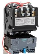
Non-reversing motor starter Size 2 Three phase full voltage Solid-state overload relay OLRelay amp range 13-52a 110VAC 50HZ / 120VAC 60HZ coil Combination type No enclosure
