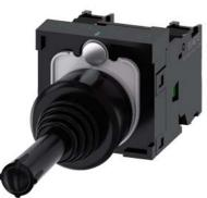
Coordinate switch, 22 mm, round, plastic, black, 2 switch positions, vertical, momentary contact type, without mechanical interlocking in O position, with holder, 1 NO, 1 NO, screw terminal, with laser labeling, lower case
