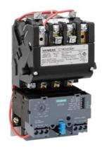
Non-reversing motor starter, Size 00, Three phase full voltage, Solid-state overload relay, OLRelay amp range 0.75-3.4a, 380 440/440 480V 50/60HZ coil, Non-combination type, Enclosure type (open), No enclosure
