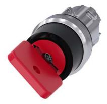
Key-operated switch O.M.R, 22 mm, round, metal, shiny, lock number 73037, red, with 2 keys, 2 switch positions O-I, latching, actuating angle 90°, 10:30h/13:30h, key removal O, with laser labeling, inscription or symbol Customer-specific selection with SIRIUS ACT configurator (CIN)
