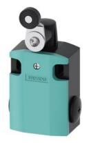
Position switch Metal enclosure 56 mm wide Device connection  $3x \, (M20x \, 1.5) \, 1$  NO/1 NC quick action contacts Rotary actuator right/left adjustable, with metal lever 27 mm long and plastic roller 19 mm
