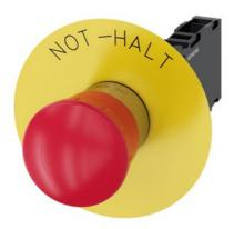
EMERGENCY STOP mushroom-type actuator, 22 mm, round, metal, shiny, red, 40 mm, positive latching, according to EN ISO 13850, rotate-to-unlatch, with yellow backing plate, inscription: NOT-HALT, with holder, 1 NO+1 NC, screw terminal
