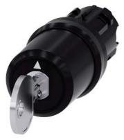
key-operated switch Siemens, 22 mm, round, plastic, lock number SSG10, with 2 keys, 3 switch positions I>O<II, momentary contact type, actuating angle 2x45°, 10:30h/12h/13:30h, key removal O Z=50-unit packaging
