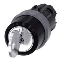
RONIS key-operated switch, 22 mm, round, plastic with metal front ring, lock number SB30, with 2 keys, 3 switch positions I>O<II, momentary contact on the left, latching on the right, actuating angle 2x45°, 10:30h/12h/13:30h, key removal O, possible special locks: SB31, 421, 455, with laser labeling, inscription or symbol Customer-specific selection with SIRIUS ACT configurator (CIN)
