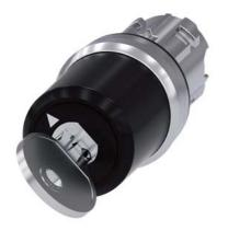
Key-operated switch BKS, 22 mm, round, metal, shiny, Lock No. E7 (VW), without key, 2 switch positions O-I, latching, actuating angle 90°, 10:30h/13:30h, key removal O+I, with laser labeling, lower case
