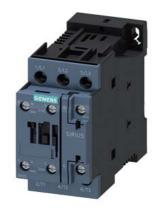
power contactor, AC-3e/AC-3, 25 A, 11 kW / 400 V, 3-pole, 24 V DC, auxiliary contacts: 1 NO + 1 NC, screw terminal, size: S0  $\,$
