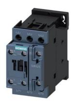
power contactor, AC-3e/AC-3, 25 A, 11 kW / 400 V, 3-pole, 230 V AC, 50 Hz, auxiliary contacts: 1 NO + 1 NC, screw terminal, size: S0, upright mounting position
